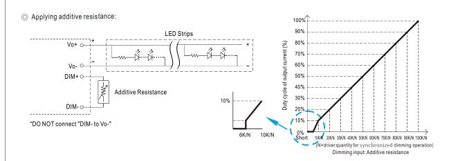
Note: 1. Min. duty cycle of output current is about 0.15%, and the dimming input is about  $6K\Omega$  or 0.6VDC, or 10V PWM signal with 6% duty cycle. 2. The duty cycle of output current could drop down to 0% when dimming input is less than  $6K\Omega$  or less than 0.6VDC, or 10V PWM signal with duty cycle less than 6%.
