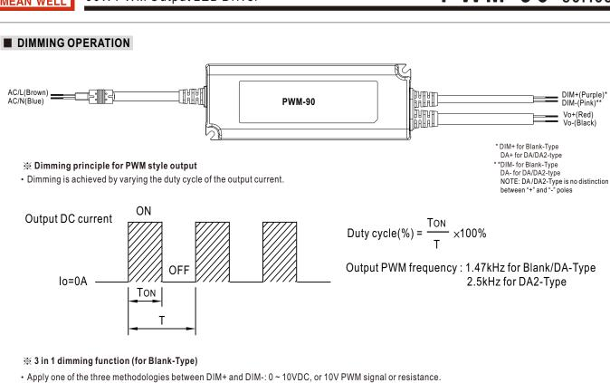
• Dimming source current from power supply:  $100\mu A$  (typ.)
