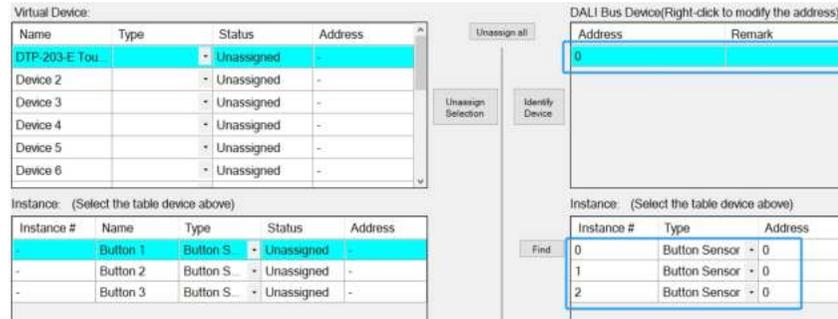
Use the mouse to select the instance number on the right area and drag it to the Virtual Device Instance position on the left area to complete the button pairing.
