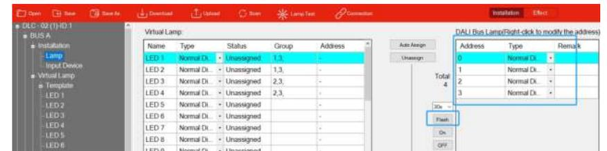
According to the actual positions of the lamps, use the mouse to select the DALI lamps on the right area, and drag them to the corresponding positions of the Virtual Lamp on the left area to complete the pairing.
