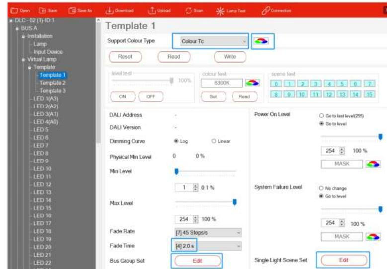
Click the colour icon and set the lamp colour temperature range to 2600–6500K (this colour temperature range is the specification of the LCM-40TW driver).
