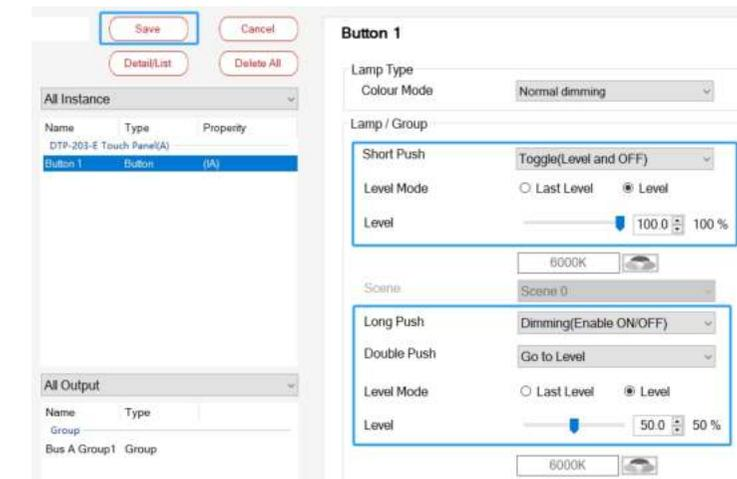
Continue to add two more effects. Refer to the configuration method for Button 1 above to complete the configuration of the control effects for "Button 2" and "Bus A Group 2", as well as "Button 3" and "Bus A Group 3".
