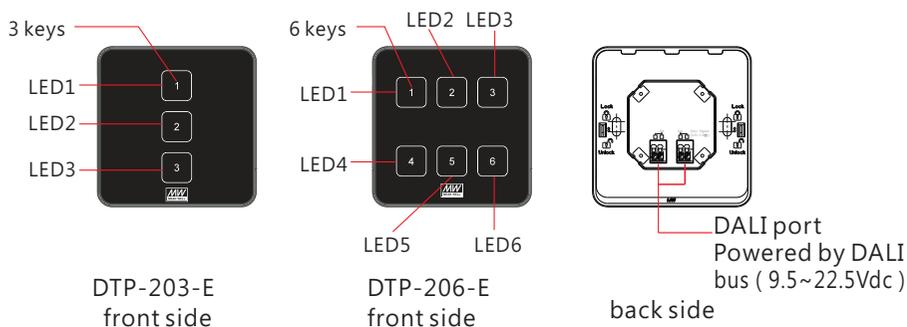
The DTP-2XX series touch panels, as input devices, are integrated into lighting control systems compliant with the DALI-2 standard. When button actions occur (e.g., short press /double press /long press, etc.), different input event commands are generated. These commands can be received and responded by other controllers on the DALI bus, which then issue corresponding control commands to adjust the state of the lamps.
