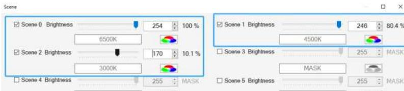
After the above parameter settings, click "**Bus A - Virtual Lamp - Template**", select **Bus A** and the "**Template 1**". In the virtual lamps table below, click "**set**" at LED 1 to LED 4 to complete the lamp parameter configuration.
