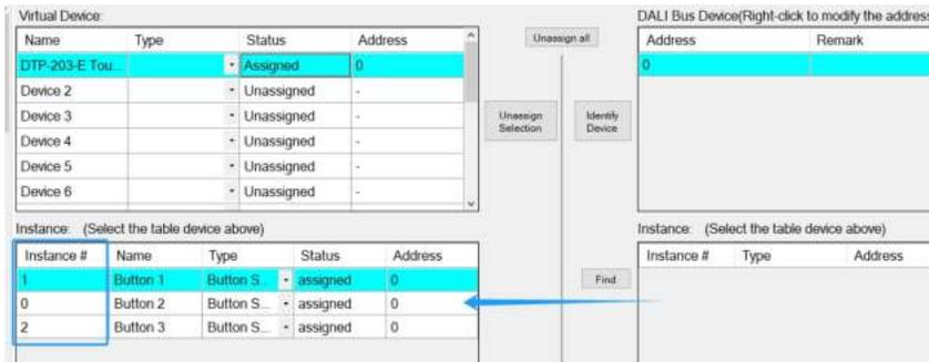
Step 5: Finally, click "Download – Device Parameter and Effect" to download all device parameters and effect configurations to the lamps, input devices, and the DLC-02 controller. After the download is complete, you can use the DTP-203-E touch panel to control the lighting changes in the conference room.
