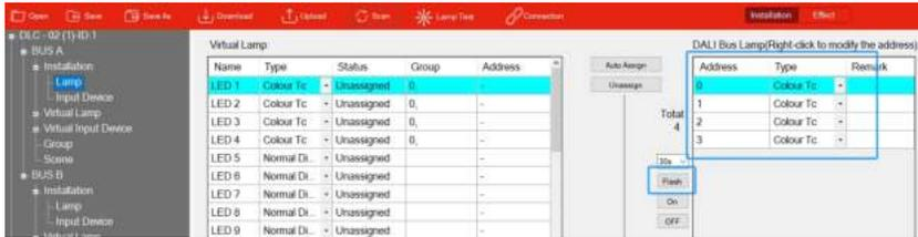
According to the actual positions of the lamps, use the mouse to select the DALI lamps on the right area, and drag them to the corresponding positions of the Virtual Lamp on the left area to complete the pairing.
