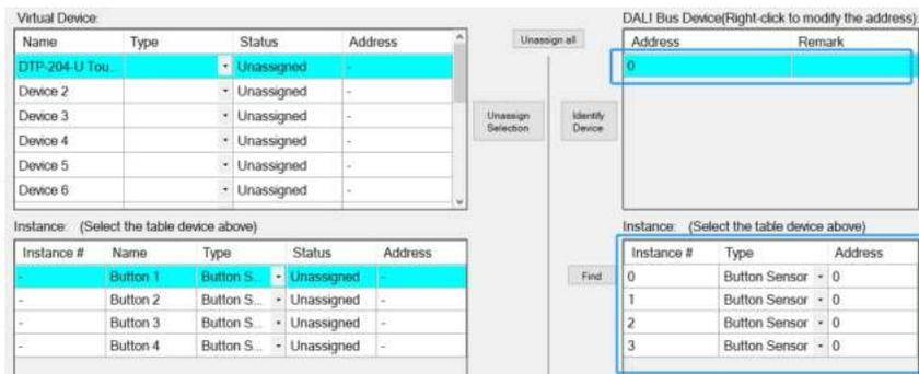
Use the mouse to select the instance number on the right area and drag it to the Virtual Device Instance position on the left area to complete the button pairing.
