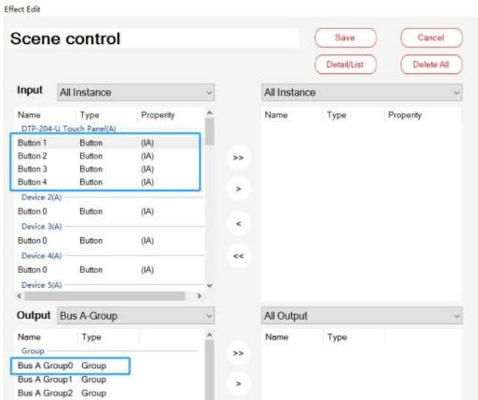
As shown in the figure, configure the control parameters for **Button 1** to **Button 4** respectively (including controlled lamp colour type, short-press execution effects, scene, brightness, colour temperature and other parameters). Click "Save" to complete the effect configuration.
