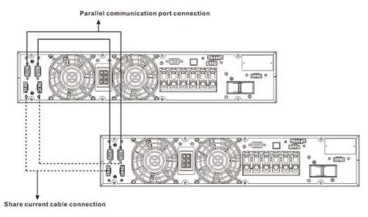
Diagram 2: Wiring diagram of parallel system
