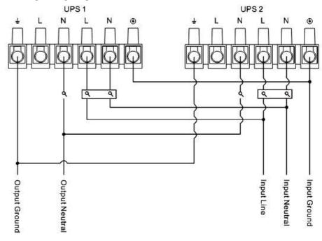
Diagram 1: Power cable connection for UPS
