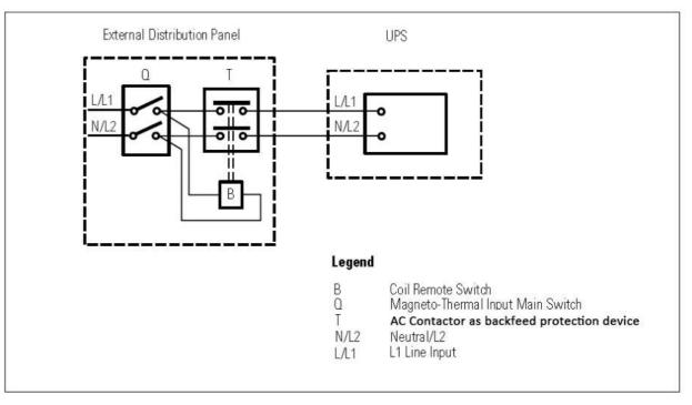
Diagram 1: External backfeed protection wiring
